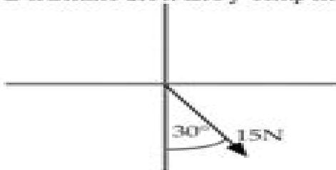
3. Write the equations for the sum of the forces acting in the x and y directions for the junction of the cords in the diagram below.
