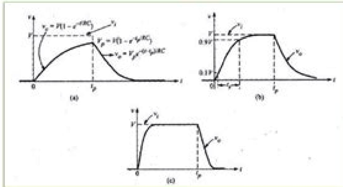
Pulse response for (a)  $RC \gg t_p$ , (b)  $RC < t_p$ , and (c)  $RC \ll t_p$
