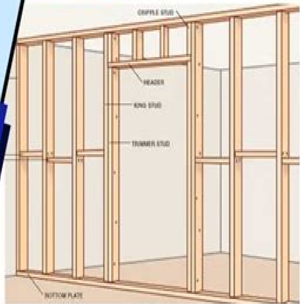
FRAMING OF AN INTERIOR WALL
