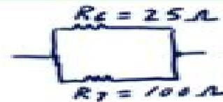
$$R_{6,7} = \frac{1}{\frac{1}{R_6} + \frac{1}{R_7}} = \frac{1}{\frac{1}{25\Omega} + \frac{1}{100\Omega}} = \frac{1}{\frac{5}{100\Omega}}$$
