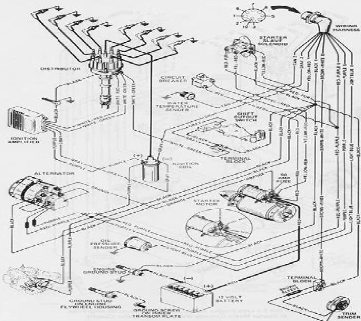
MCM 200 5.0 Litre Engine with 90 Amp Fuse at Starter Motor
